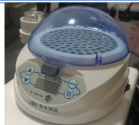
Manila HealthTek's Lab-in-a-Mug, utilized to perform all LAMP assay experiments done by the project.
