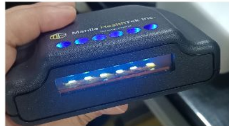
Transilluminator utilized by the project to visualize QUASR-LAMP results.
