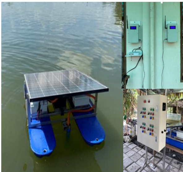
i-POND: LoRaWAN-based Pond Water Quality Control and Monitoring System for Shrimp Farms
